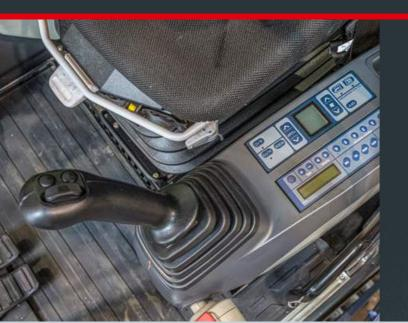
A key feature of the SY135C is comprehensive comfort for its drivers. Excellent insulation around the cab provides reliable protection from noise and vibrations, as well as from high and low temperatures. The air-suspension driver's seat, provided as standard, offers the best possible comfort and protection from fatigue with its high seat backrest and various adjustment options.
